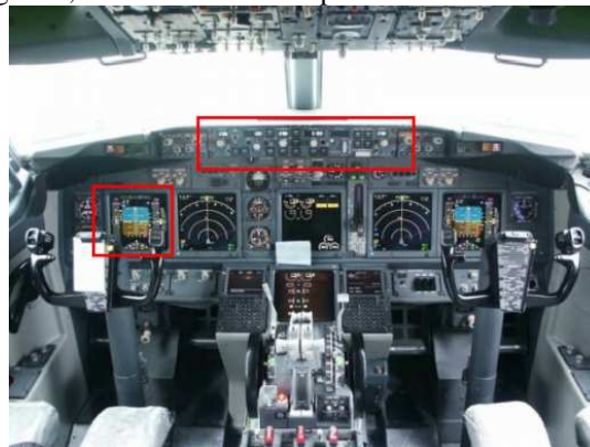
Fig 4 Aircraft cockpit [9], pilot’s AP/FP Mode Control Panel (detail in figure 5), pilot’s primary flight display - PFD (detail in figure 6)
