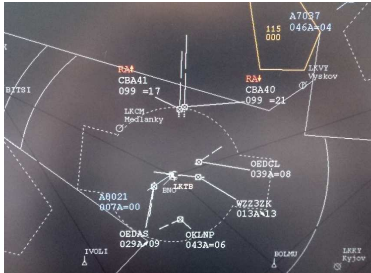
Fig 9 Radar screen from 13 May 2013 where is depicted “RA” warning in labels of inspection flights CALIBRA40 and CALIBRA41 during testing new primary radar installed in LKTB. (Both aircraft are closer to each other than prescribed separation minima (5, resp. 3 NM horizontally and 1000ft vertically))
