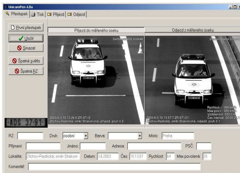
Fig. 2: Photo at entry of measured section (left) and the same car at exit (right). The recognized license plate is on left hand site
