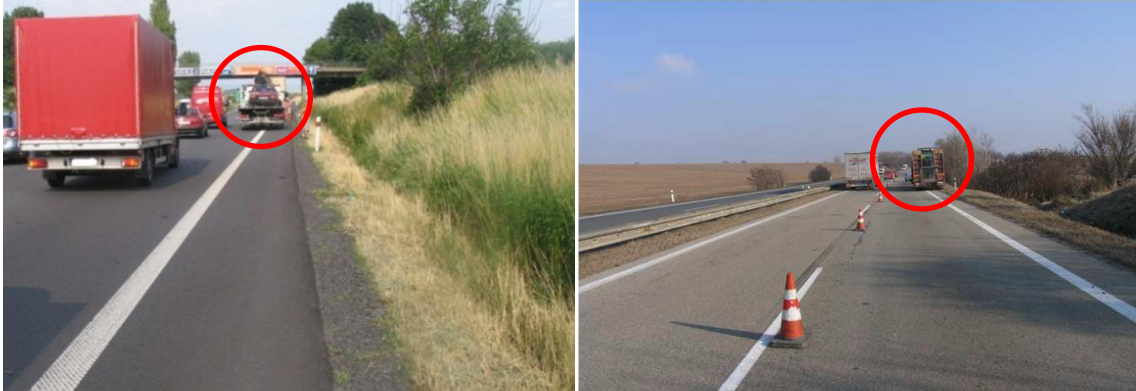
Fig. 14. Problem 8 – Vehicle pulled aside still significantly covers the main traffic lane
