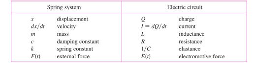
We can also transfer other ideas from one situation to the other. For instance, the steady state solution discussed in Note 1 makes sense in the spring system. And the phenomenon of resonance in the spring system can be usefully carried over to electric circuits as electrical resonance.
