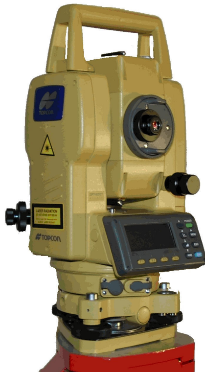
obr. 7 Total-Station TOPCON GPT 3007
